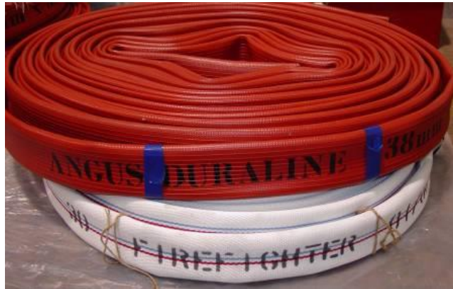
Figure 3 – Suggested Damaged Hose Marking Method
