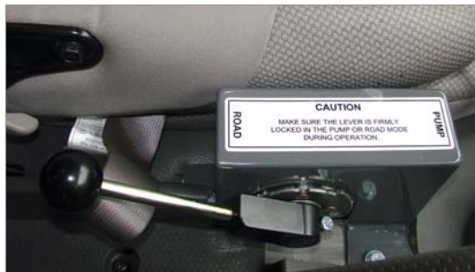
Figure 2 – power take off lever
