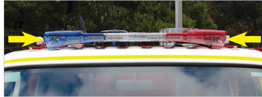
Figure 14 – alley lights in LED roof bar
