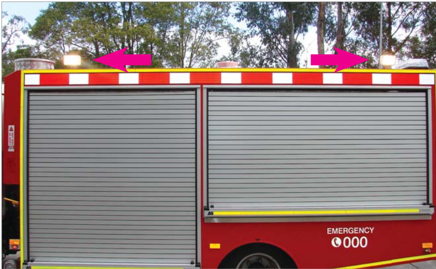
Figure 21 – near side work lights
